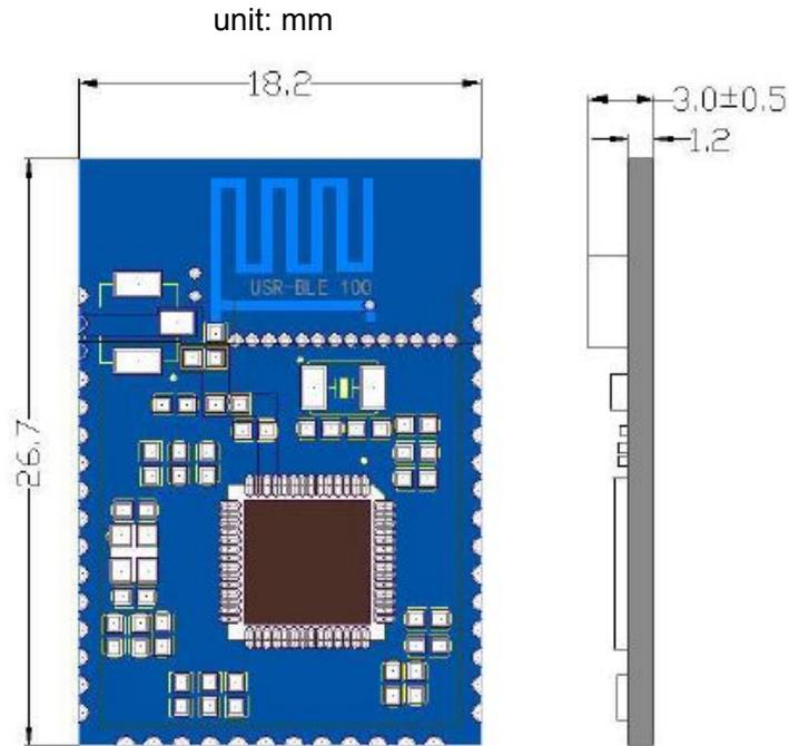
**Figure 5 USR-BLE100 Dimension**
