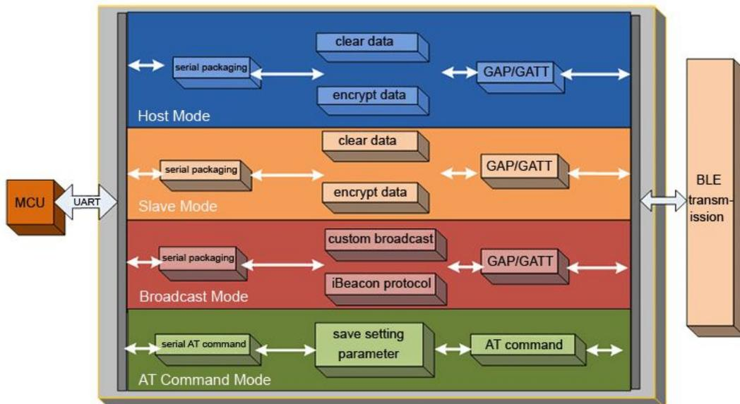
**Figure 6 USR-BLE100 Function**
