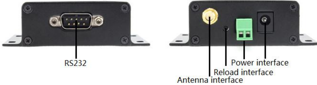
Figure 6 USR-WIFI232-602 V2 interface
